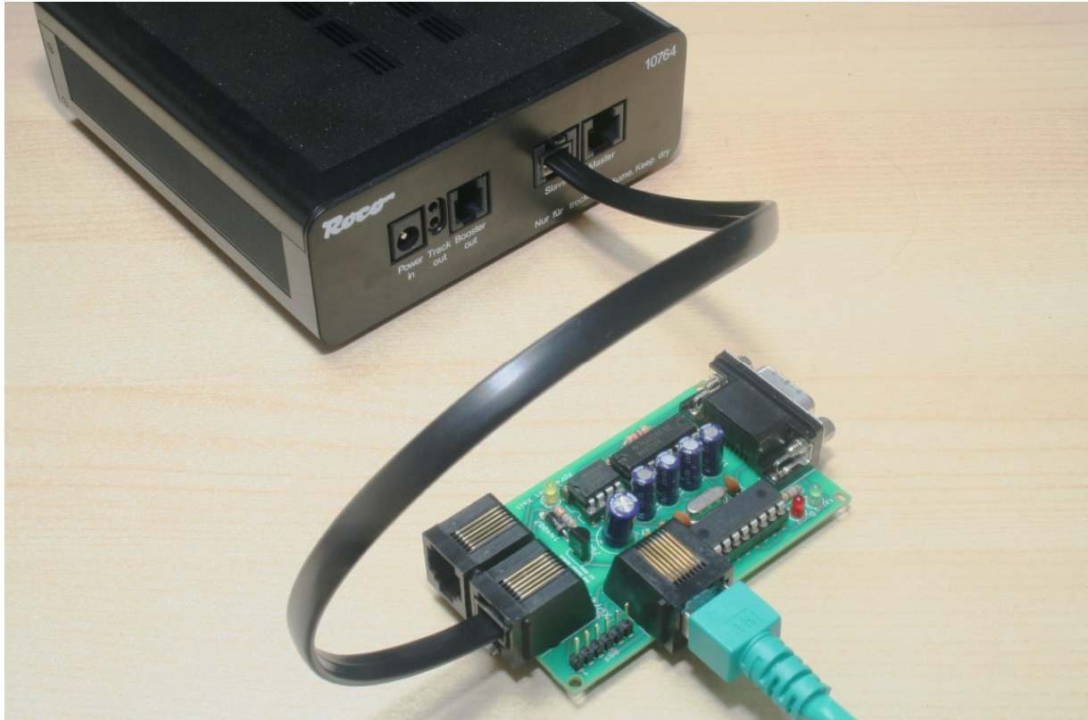
Picture showing the connection of the S88XPressNetLI to the ROCO® amplifier's SLAVE port, note that also the s88-N port has been connected.
